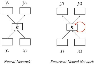
**Figure 1:** On the left, an artificial neural network. On the right, a recurrent neural network. Both architectures have two inputs, two outputs and a single hidden unit.
