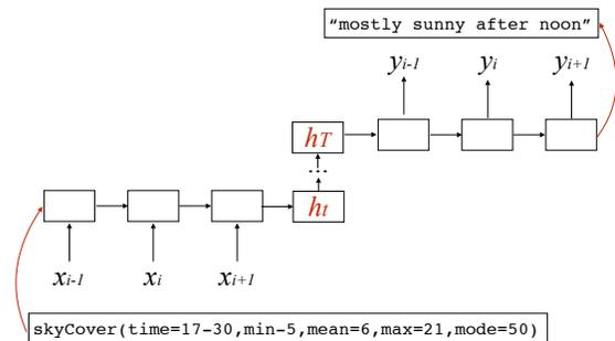
**Figure 8:** Sequence-to-sequence LSTM learning a mapping from an input sequence  $\mathbf{x}$  of meteorological measurements to an output sequence  $\mathbf{y}$  of words.
